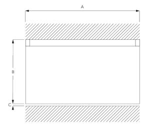
A: System width B: System height C: Distance between floor and fabric
