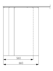
2 panels: 560 mm 3 panels: 660 mm 4 panels: 760 mm
